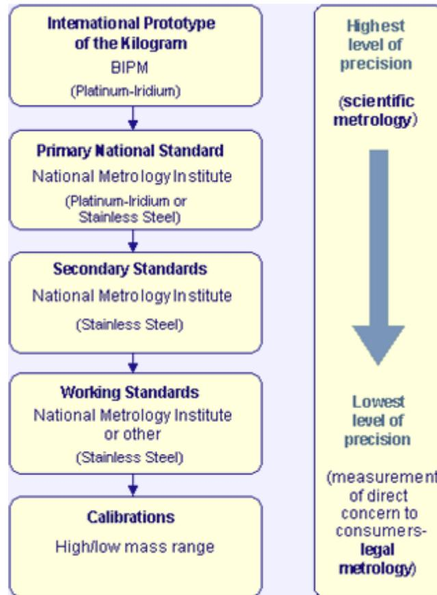
Fig. 1.5: Types of standards that exist in a particular area of metrology
