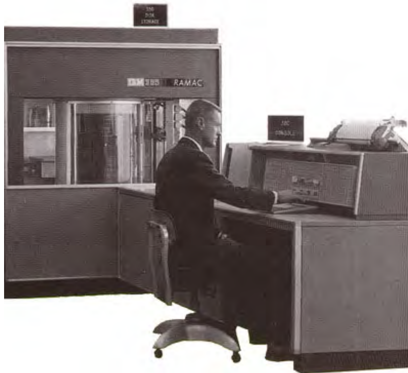
Fig. 7.7: RAMAC, the first magnetic disk storage device
