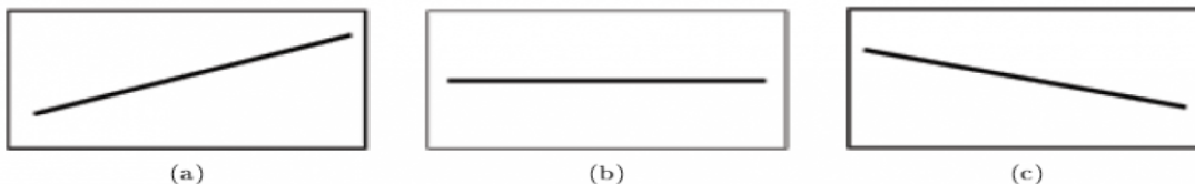
Figure 6.2 Three possible graphs of y = a + bx . (a) If b > 0 , the line slopes upward to the right. (b) If b = 0 , the line is horizontal. (c) If b < 0 , the line slopes downward to the right.
