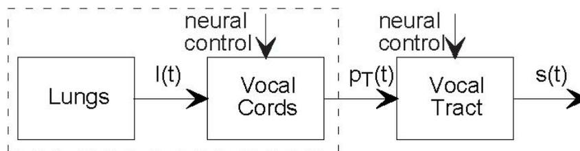
**Figure 4.14 Model of the Vocal Tract** The systems model for the vocal tract. The signals  $l(t)$ ,  $p_T(t)$ , and  $s(t)$  are the air pressure provided by the lungs, the periodic pulse output provided by the vocal cords, and the speech output respectively. Control signals from the brain are shown as entering the systems from the top. Clearly, these come from the same source, but for modeling purposes we describe them separately since they control different aspects of the speech signal.
