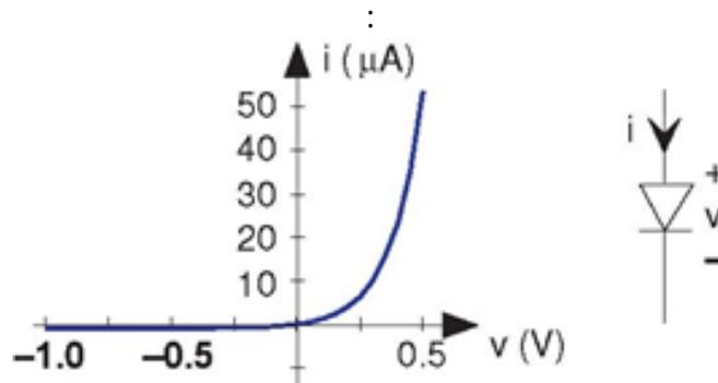
**Figure 3.48** Diode  $v$ - $i$  relation and schematic symbol for the diode. Here, the diode parameters were room temperature and  $I_0 = 1 \mu A$ .
