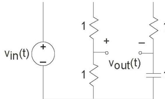
Figure 4.20 Phase Distortion
