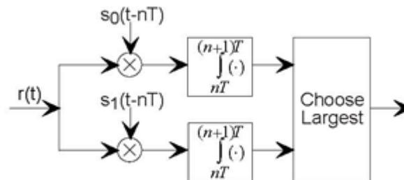
Figure 6.14 Optimal receiver structure
