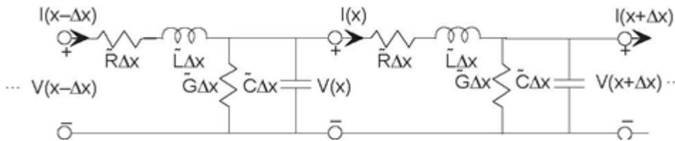
Figure 6.2 Circuit Model for a Transmission Line
