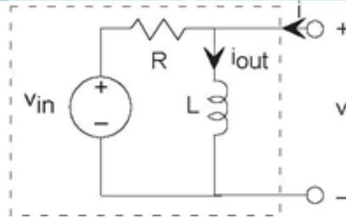
Figure 3.31 RL circuit
