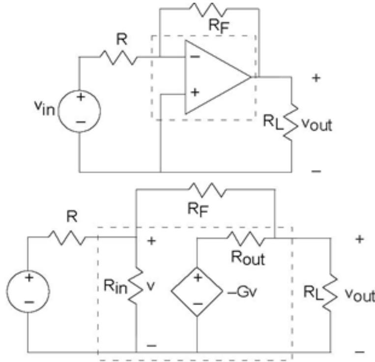
**Figure 3.43 op-amp 2** The top circuit depicts an op-amp in a feedback amplifier configuration. On the bottom is the equivalent circuit, and integrates the op-amp circuit model into the circuit.
