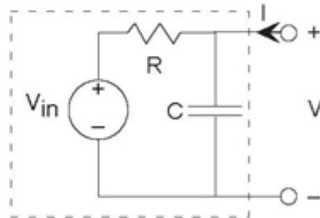
Figure 3.28 Simple RC Circuit
