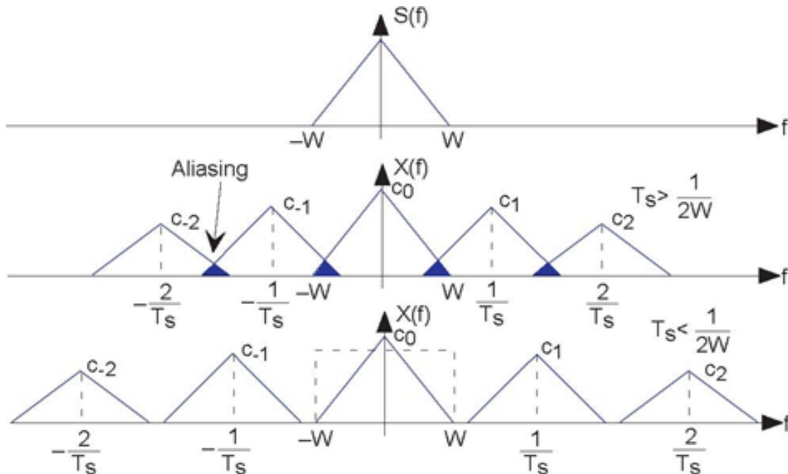
**Figure 5.4 aliasing** The spectrum of some bandlimited (to  $W$  Hz) signal is shown in the top plot. If the sampling interval  $T_s$  is chosen too large relative to the bandwidth  $W$ , aliasing will occur. In the bottom plot, the sampling interval is chosen sufficiently small to avoid aliasing. Note that if the signal were not bandlimited, the component spectra would always overlap.
