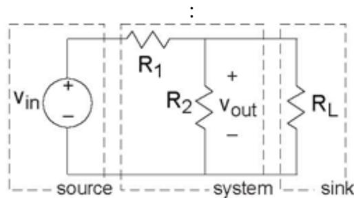
Figure 3.13 Circuit example 3 The simple attenuator circuit is attached to an oscilloscope's input. The input-output relation for the above circuit without a load is:
