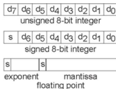
**Figure 5.2 Number representations on computers** The various ways numbers are represented in binary are illustrated. The number of bytes for the exponent and mantissa components of floating point numbers varies.
