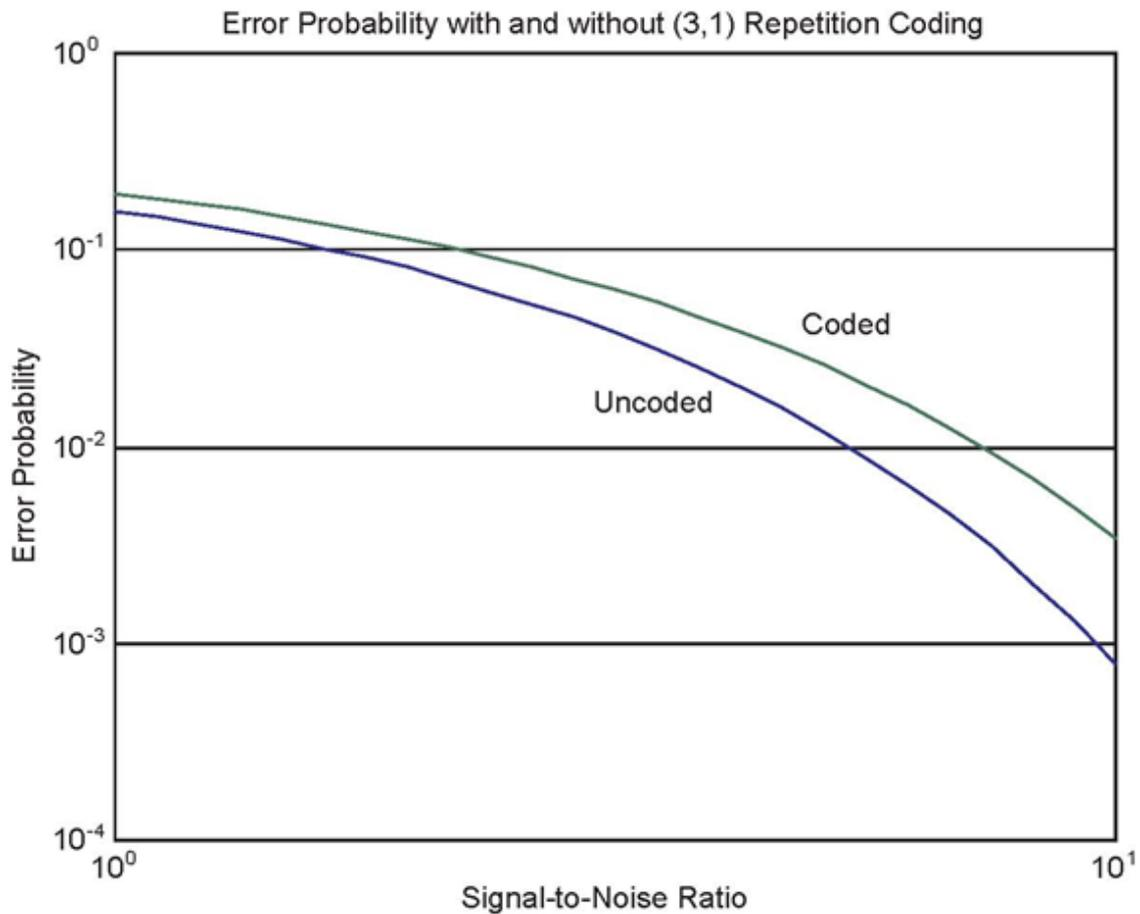
Figure 6.44 Error Probability with and without (3,1) Repetition Coding
