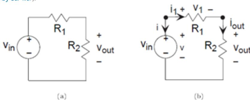
**Figure 3.8 Circuit examples** The circuit shown is perhaps the simplest circuit that performs a signal processing function. The input is provided by the voltage source  $v_{in}$  and the output is the voltage  $v_{out}$  across the resistor labelled  $R_2$
