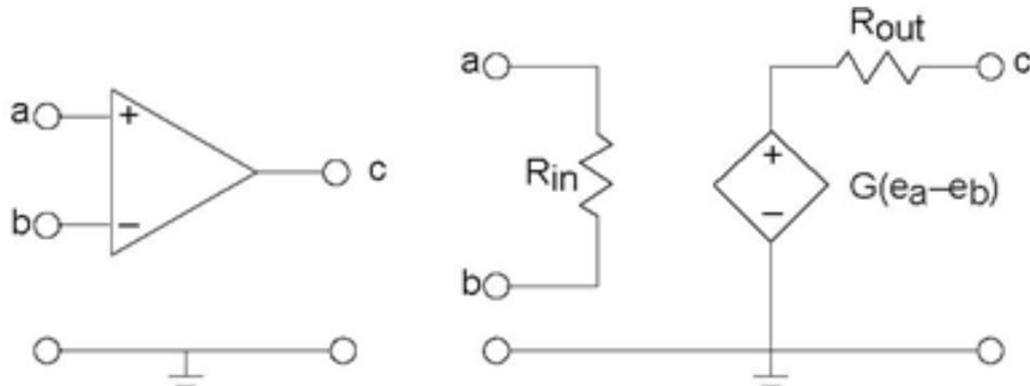
**Figure 3.40 op-amp** The op-amp has four terminals to which connections can be made. Inputs attach to nodes a and b, and the output is node c. As the circuit model on the right shows, the op-amp serves as an amplifier for the difference of the input node voltages.
