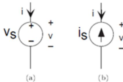
**Figure 3.5 Sources** The voltage source on the left and current source on the right are like all circuit elements in that they have a particular relationship between the voltage and current defined for them. For the voltage source,  $v = v_s$  for any current  $i$ ; for the current source,  $i = -i_s$  for any voltage  $v$
