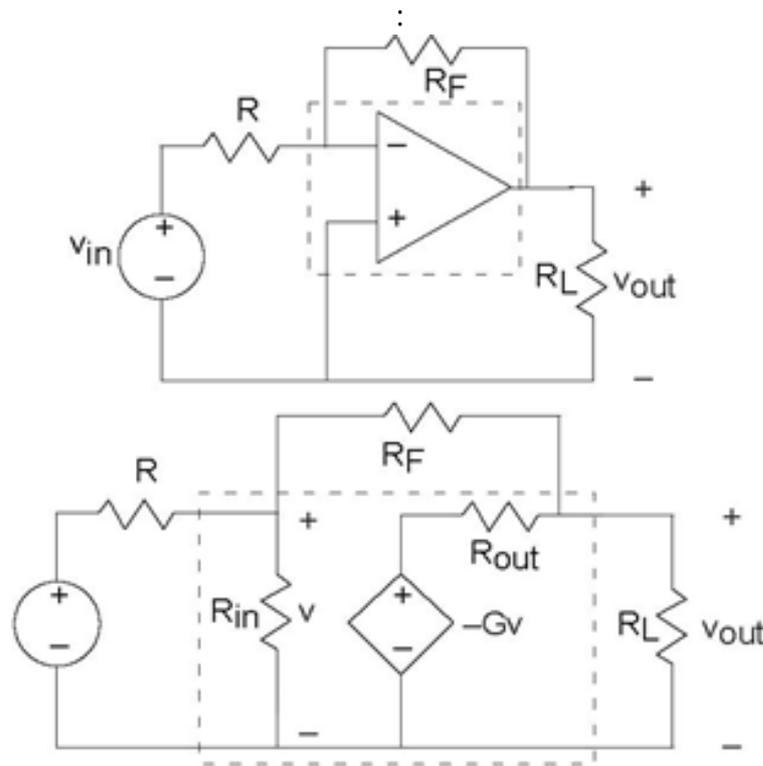
**Figure 3.41 feedback op-amp** The top circuit depicts an op-amp in a feedback amplifier configuration. On the bottom is the equivalent circuit, and integrates the op-amp circuit model into the circuit.
