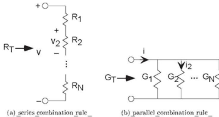
Figure 3.15 Series and parallel combination rules
