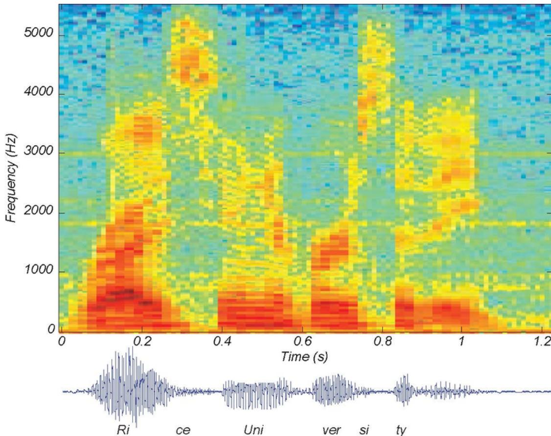
**Figure 4.17 spectrogram** Displayed is the spectrogram of the author saying "Rice University." Blue indicates low energy portion of the spectrum, with red indicating the most energetic portions. Below the spectrogram is the time-domain speech signal, where the periodicities can be seen.
