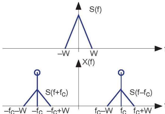
**Figure 4.12 Spectrum of the amplitude modulated signal** A signal which has a triangular shaped spectrum is shown in the top plot. Its highest frequency the largest frequency containing power is  $W$  Hz.
