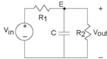
**Figure 3.36 Node Method and Impedances** Modification of the circuit shown on the left to illustrate the node method and the effect of adding the resistor  $R_2$ .
