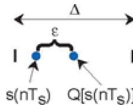
**Figure 5.6 A single quantization interval** A single quantization interval is shown, along with a typical signal's value before amplitude quantization  $s(nT_s)$  and after  $Q(s(nT_s))$ .  $E$  denotes the error thus incurred.
