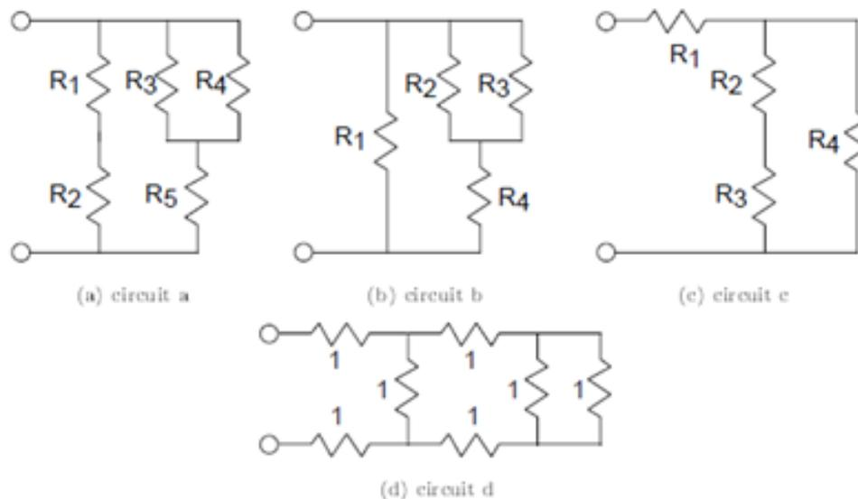
Figure 3.54 Equivalent Resistance
