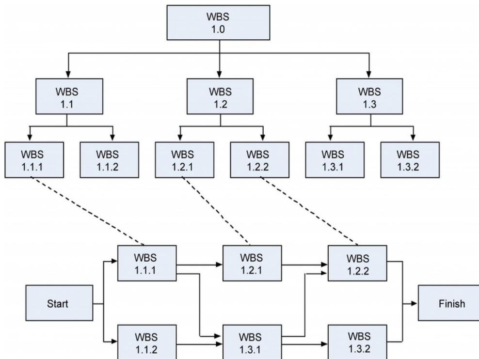
**Figure 10.10** An example of an activity on node (AON) diagram. Illustration from Barron & Barron
