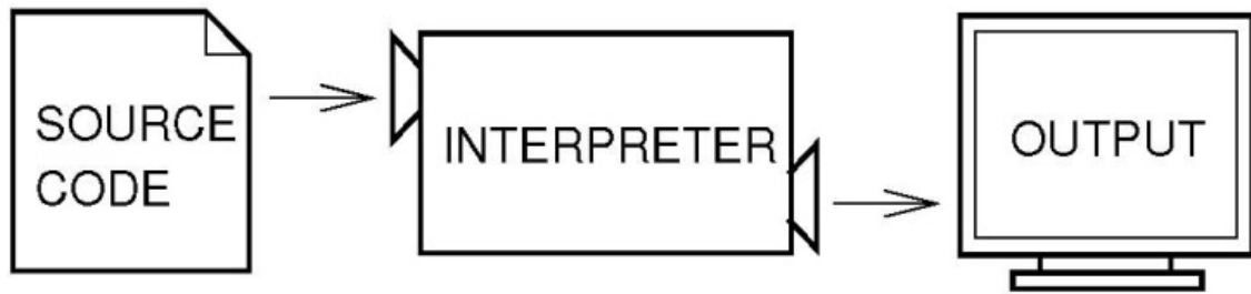
Fig. 1.1: An interpreter processes the program a little at a time, alternately reading lines and performing computations
